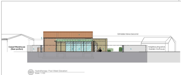
124.1 Hydrotherapy Pool West Elevation Scale: 1:100
